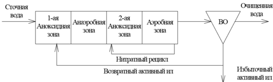
Fig. 2.53 - Schematic diagram of the JHB process
