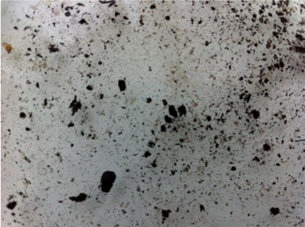
Fig. 11a – photo of particles of contaminants in water without treatment with reagents.
