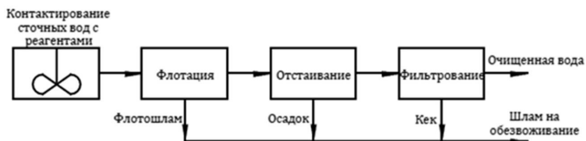
Fig. 2.18. Scheme of water purification in the flotical combine
