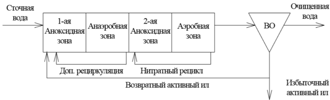
Fig. 2.54 - Schematic diagram of the modified JHB process
