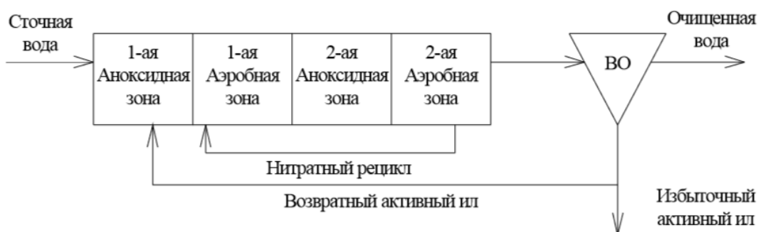
Fig. 2.51 - Schematic diagram of the Bardenpho process
