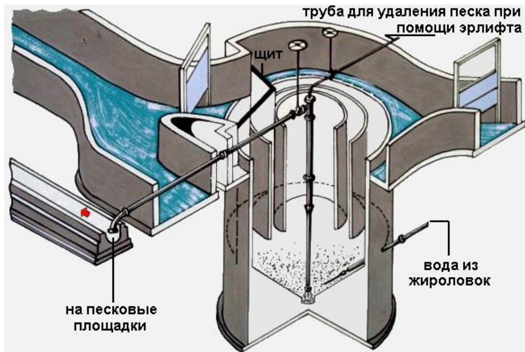
Fig. 2.4 - Scheme of water movement in a sand trap
