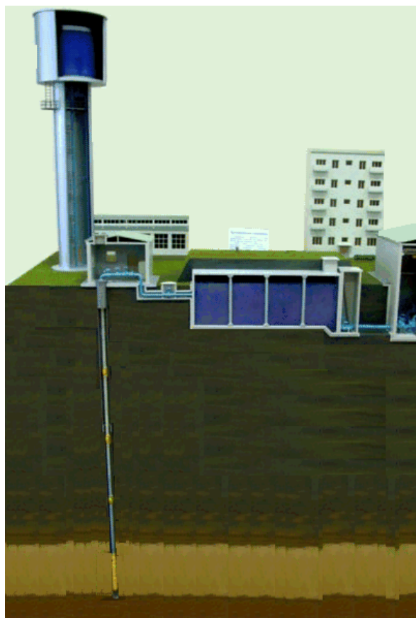
Fig. 1.5. Scheme of water supply from an underground source
