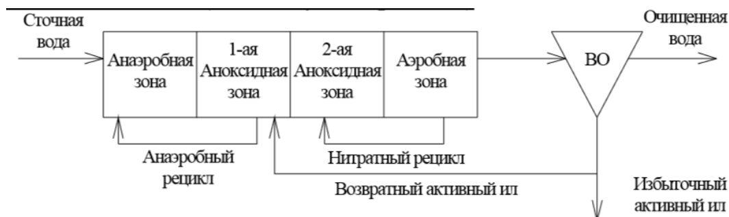
Fig. 2.50 - Schematic diagram of the Modified UCT process
