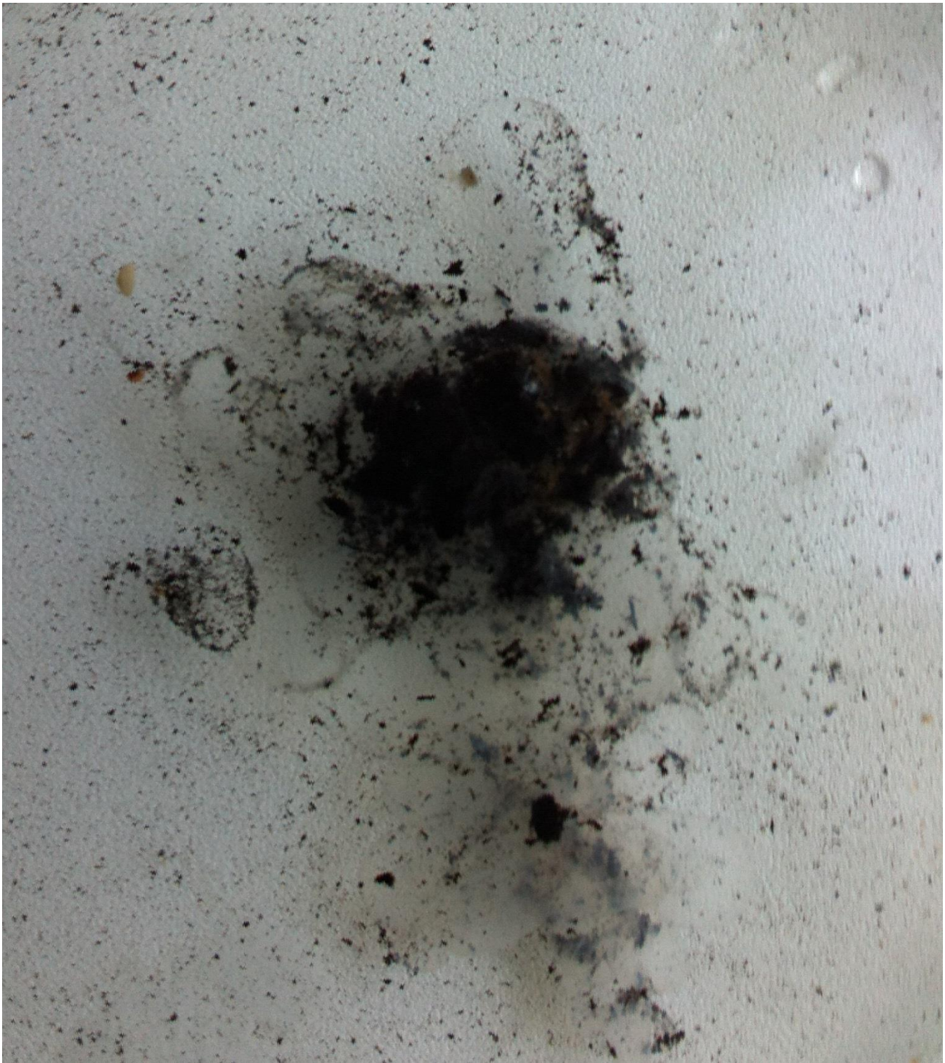
Fig. 11b – photo of pollution particles in the form of large aggregates after adding aluminum sulfate and flocculant praestol 655 to water
