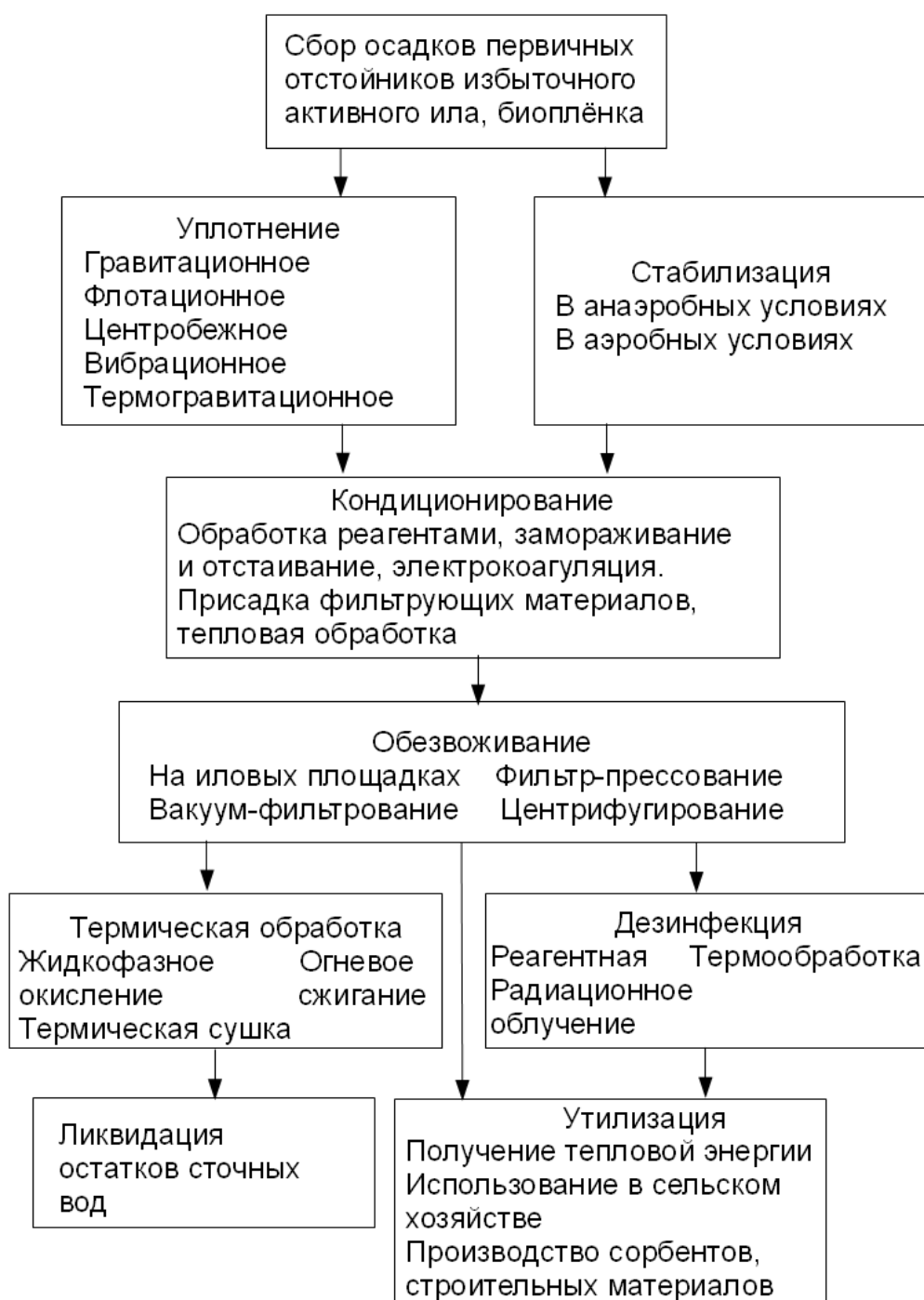
Fig. 2.58 - Methods and processes used in the treatment, disposal and disposal of sewage sludge
